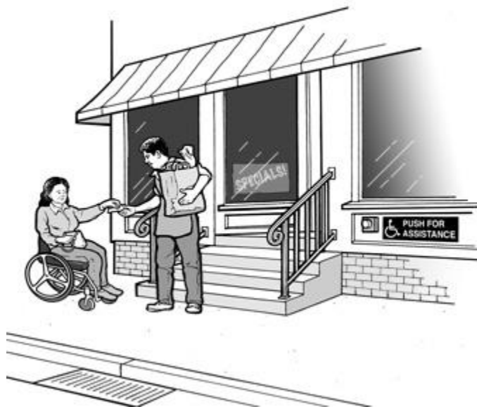
When barrier removal is not possible, alternatives such as curbside service should be provided.
